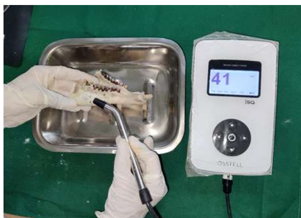
Fig No.5: Primary stability of each mini-implant measured using Osstell ISQ on Jaw 1 and 2.
